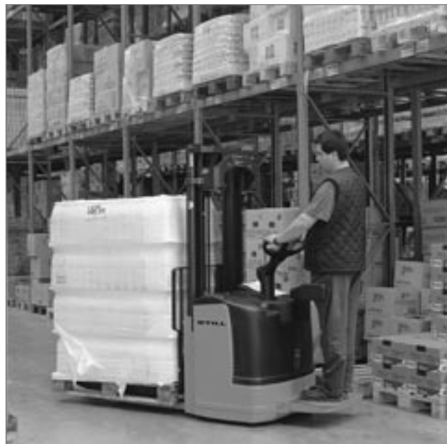
The EGV-S is particularly suitable for longer runs due to the hinge-down stand-on platform.
