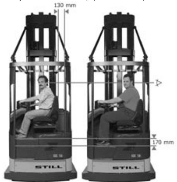
GX/Q 13 Adjustment of the driver's seat proportional to the floor plate.
