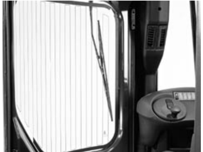
Feel comfortable - even in bad weather with a weather protection cab including heated screens and screen washer for outdoor use.
