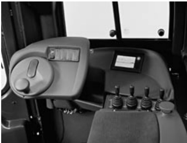
The ergonomic driver's compartment with four individual fingertip control levers for sensitive hydraulic functions
